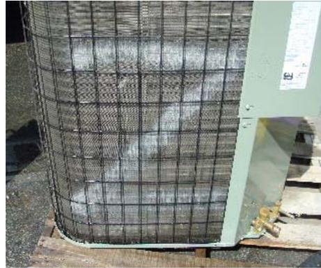
Here's what a pressure sprayer does to a standard coil!
